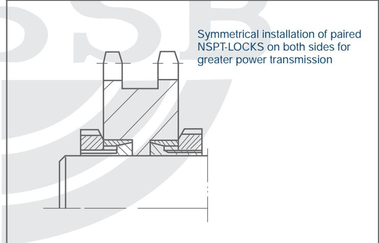
Symmetrical installation of paired NSPT-LOCKS on both sides for greater power transmission
