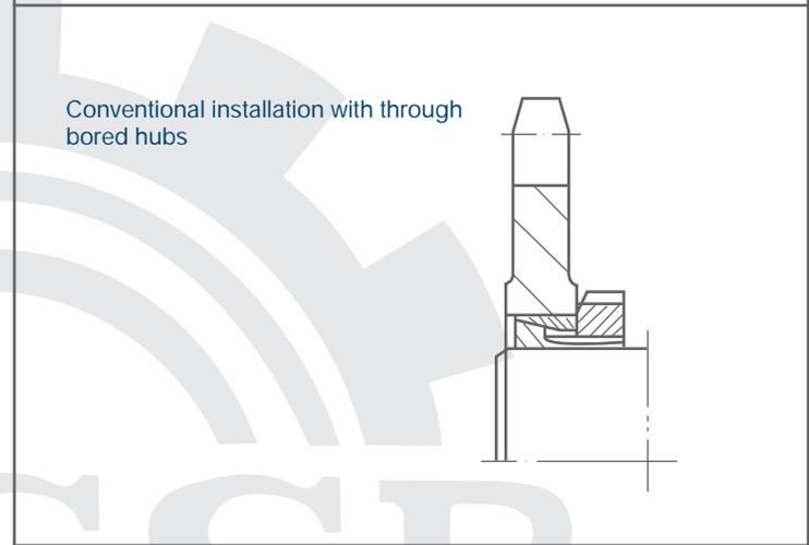
Conventional installation with through bored hubs
