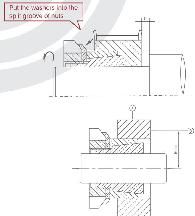
After the correct installation mentioned above inspect the runout for (A) and (B). The run out for (A) should not excess 0.05mm and 0.02mm for (B).
