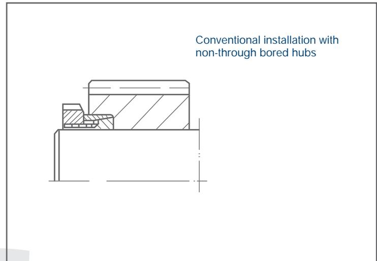
Conventional installation with non-through bored hubs
