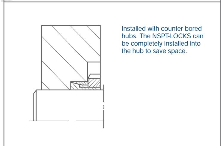
Installed with counter bored hubs. The NSPT-LOCKS can be completely installed into the hub to save space.
