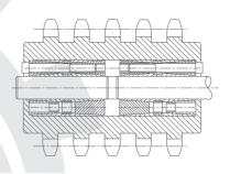
Mounted with shaft sleeves to connect transmission between two shafts. They have the same function as couplings
