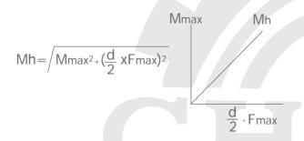
Mmax--Required transmitted torque Nm Fmax--Required transmitted axial force N Mh--synthetic transmitted torque Nm d--Transmission shaft diameter mm Mt--NSPT LOCK rated transmitted torque Nm
