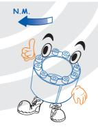
3.NSPT-LOCKS can be used and disassembled repeatly. But after each repeated installation and disassembling, the shape of NSPT-LOCKS will change slightly. Torque will be reduced slightly as well.
